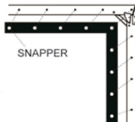
(Eng) Snap/connect the four corners of the screen fabric first, followed by long- and short sides.
