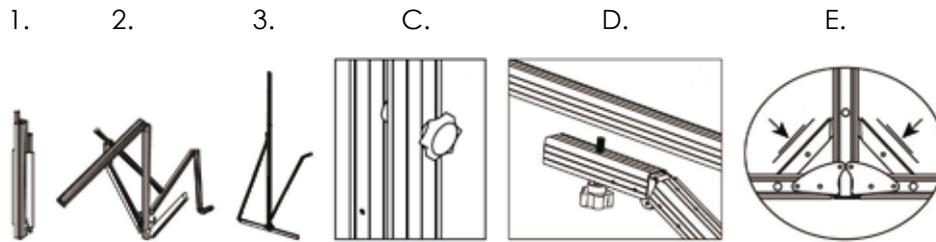
(Eng) Mount the two stands, fig 1, 2 and 3. Make sure the legs are locked, fig E. Connect the stands to the frame using the M8 knobs, fig C and D.
