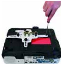
5. Projector standoffs are adjustable spacers which can be used to level the arms of the Christie One Mount. The projector standoffs also ensure screws are centered when the projector is
