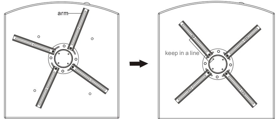
Place the projector bracket as close as possible to the projector's center of gravity. Position the holes of arms over the mounting holes.
