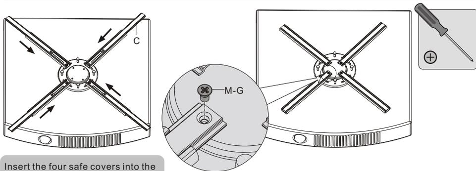
Insert the four safe covers into the arms of adapter bracket till they fit mounting hole pattern.
