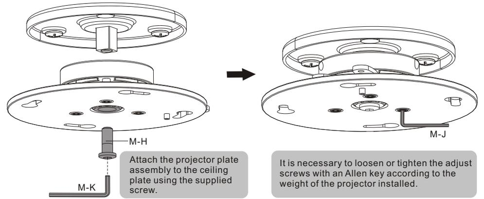
Attach the projector plate assembly to the ceiling plate using the supplied screw.
