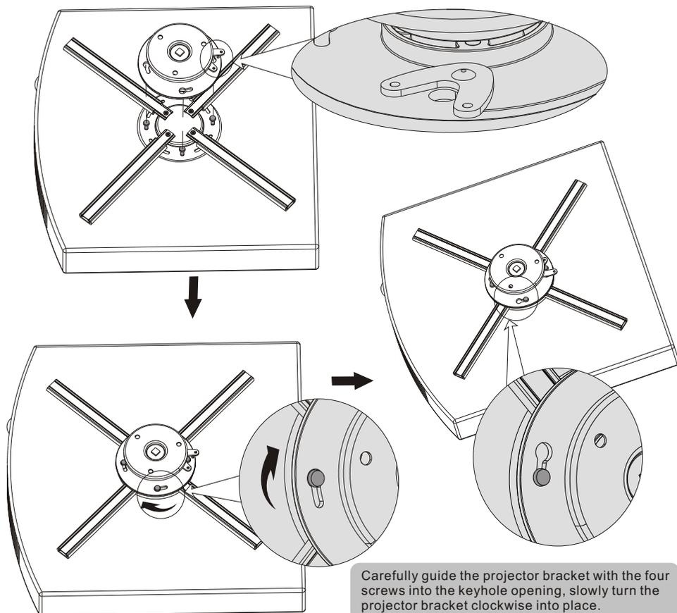
Carefully guide the projector bracket with the four screws into the keyhole opening, slowly turn the projector bracket clockwise into place.
