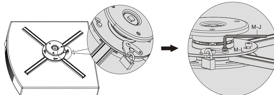
Use the padlock in the locking plate and then fix the locking plate with a screw to prevent the projector plate assembly rocking in use.
