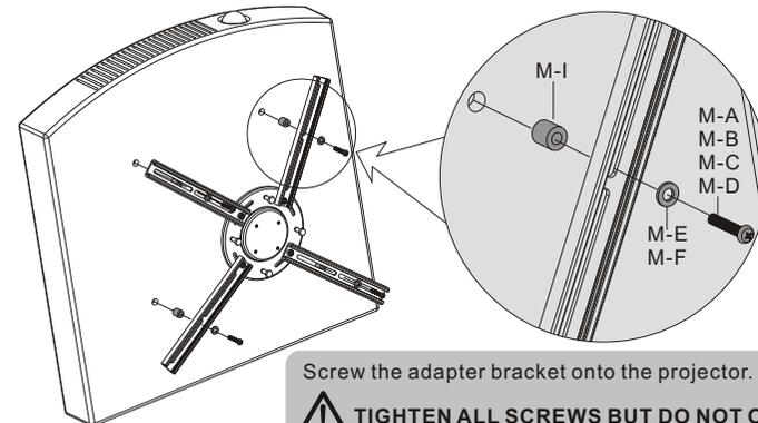
Screw the adapter bracket onto the projector.
